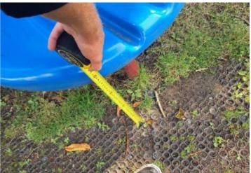
Finding: The height of the slide runout is in excess of 350mm and does not meet the requirements of BS EN 1176:
