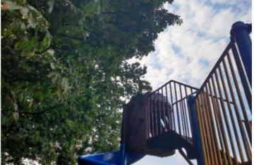
**Finding:** The tree canopy overhangs the equipment and is less than 2.0m away
