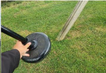
**Finding:** The seat is less than 2.0 metres from the post when extended at 45 degrees at the end of the area of travel minimum distance is maintained and does not meet the requirements of BS EN 1176 Part 4
