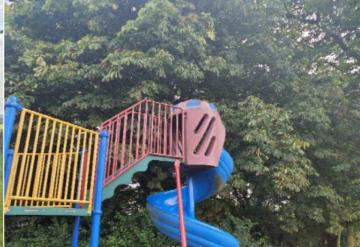
**Finding:** This item of equipment has a fall height in excess of 2.5m and grass mats have been installed as an impact absorbing surface; these mats rely heavily on the underlying surface to achieve their critical fall height properties.
