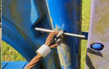
Finding: The connecting links are in excess of 8.6mm and less than 12mm and fail the requirements of BS EN 1176 Part 1; clause 4.2.13, Chains
